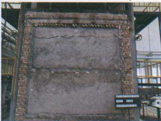
照片 2. 试验前试件背火面情况 Condition of surface unexposed to fire before testing.
