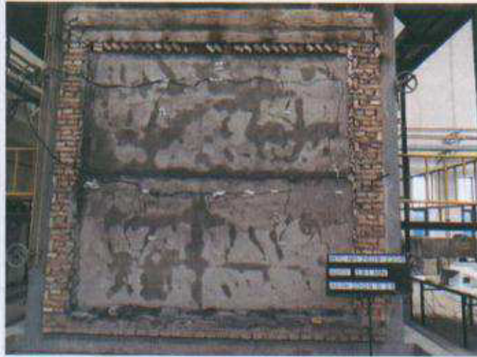
照片 3. 试验 181min 时试件背火面情况 (Condition of surface unexposed to fire when test start 181 min).
